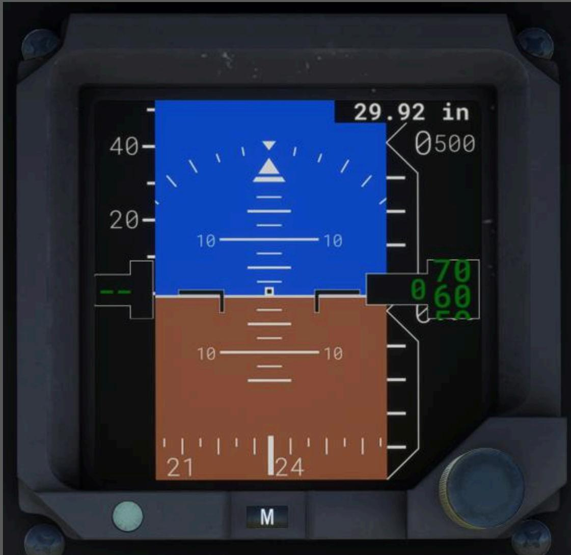
The Integrated Standby Instrument (ISI) is your backup display for key flight data—attitude, altitude, and airspeed—when the primary instruments fail. Here’s a simple breakdown of how it works and what it does:
