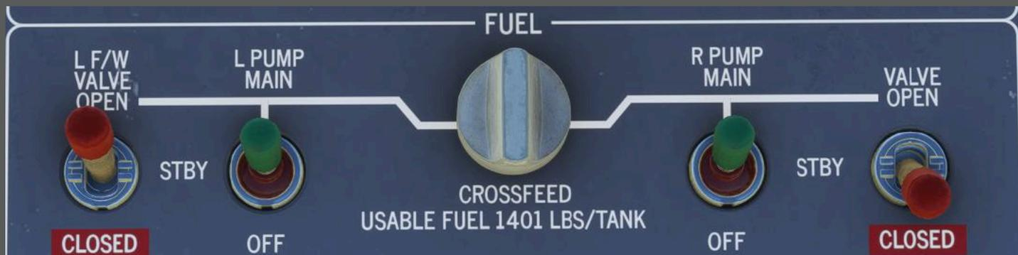
The aircraft's fuel system holds about 1,600 liters (around 420 U.S. gallons) in total, with nearly all of that being usable fuel.
