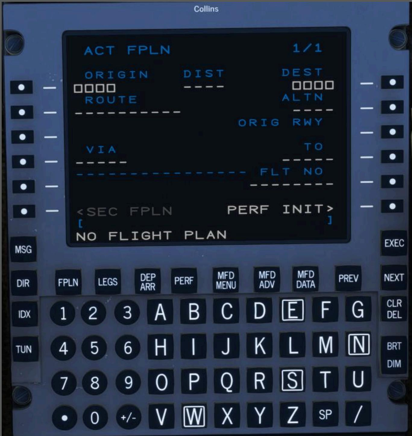
The Flight Management Computer (FMC) is a central interface on the control pedestal that lets you manage both flight planning and radio functions, such as communication, navigation, and transponder settings. Here's a simple breakdown of its features:
