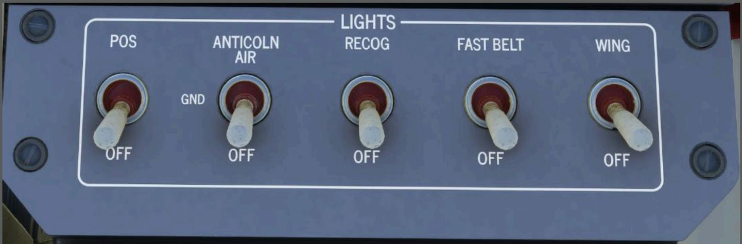
The anticollision and ground beacon lights get their power from a dedicated circuit on the copilot's panel. You control them with a three-position switch labeled "ANTI COLN AIR-GND-OFF":
