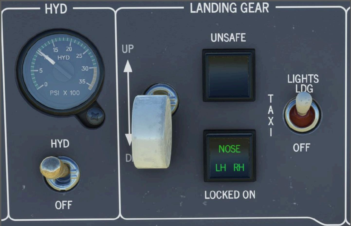
A constant tone sounds to warn you when the landing gear isn't fully down and locked, under these conditions:
