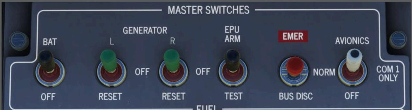
The electrical system controls are found on two panels: the MASTER SWITCHES panel on the center of the instrument panel and the ENGINE/PROPELLER panel on the control pedestal. Here's what each switch does and where it's used:
