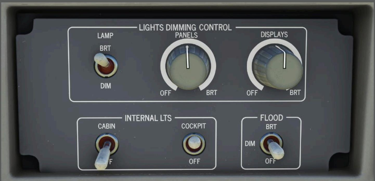
The internal lighting control panel, located on the left side of the cockpit, lets you adjust the brightness of all the cabin lights. Here's a breakdown of how it works:
