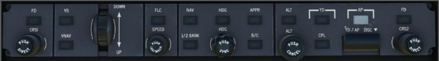
The Flight Management Computer (FMC) Flight Guidance System (FGS) is essentially your autopilot and flight director combined, which helps you fly the plane automatically or provides guidance cues. Here's a plain-language rundown of its key functions and how you use them:
