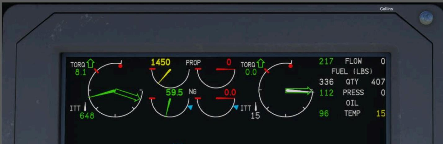
The Engine Indicating System (EIS) normally appears on the top portion of the Multifunction Display (MFD) and shows key engine data for both the left and right engines. These readings include:
